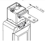
This switch has a wide backlash of the actuator into the head (4,5 mm) to avoid that door gaskets keep in traction the actuator on the solenoid. With closed door, check that the actuator doesn't knock straight against the head of the switch; it must be in the adjustment zone (0,5...5
