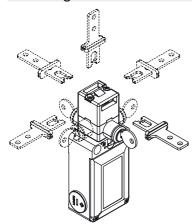
The head can be quickly rotated on each of the 4 sides of the switch by unfastening the two fixing screws. The mechanical lock release device can be rotated in 90° steps as well. This enables the switch to assume 32 different configurations.
