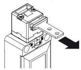
Thanks to recent mechanical improvement the strong interlocking system guarantees a maximum actuator holding force of 1100 N (head
